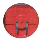
Decks are reinforced with internal 7-gauge steel strongbacks that run the full length of the deck, tying together the entire structure with the gearbox stand. Bush Hog® blade pans are round to allow the mower to float over field obstructions.
